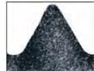
Modified thread: Note stress relieving radii in this unretouched photo enlargement of the supabuckle.
