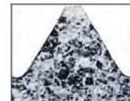
Standard thread: Note stress building sharp "V" in this untouched photo enlargement.
